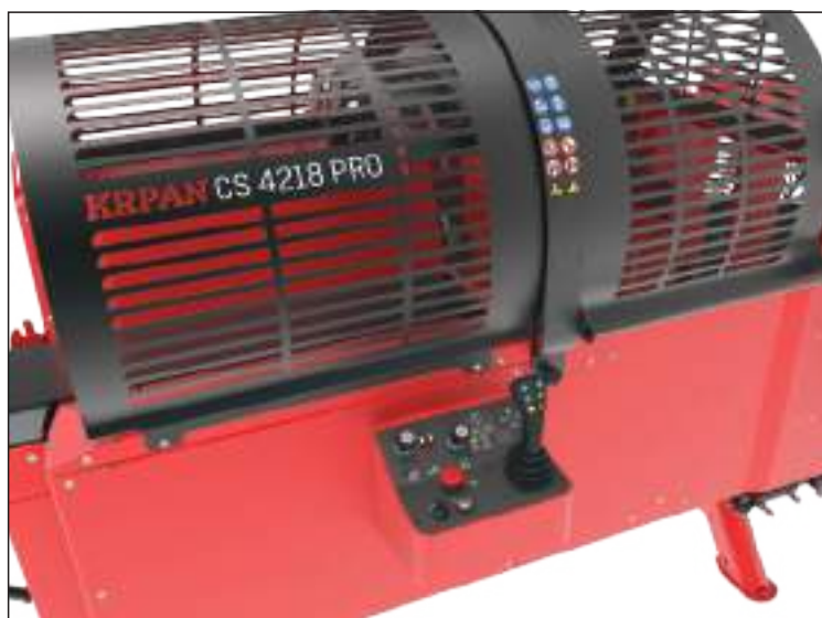
KRPAN CS 4218 PRO controlled by joystick all movements of individual assemblies are performed electro-hydraulically, except for the setting of the firewood length limiter
